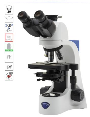
Phase contrast, darkfield and brightfield trinocular microscope with W-PLAN objectives, rackless stage and the exclusive **X-LED**<sup>3</sup> for great-looking, rich and high-quality view.
