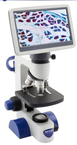
Two models of the B-60 series can be equipped with a camera and a 7" LCD screen, both in high definition. In these bundles, the normal head (supplied with the instrument) can be replaced with the digital system in a few minutes. This solution provides a system suitable for viewing specimens by several students at the same time, without removing the possibility of using the microscope in the classical way through the eyepiece.
