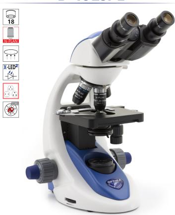
Binocular microscope ideal for teachers and secondary schools, with four N-PLAN objectives (600x), FN 18 high eyepoint, finite optical system, coaxial focusing, mechanical stage, Abbe condenser and powerful, uniform, white color temperature 3 W *X-LED*<sup>2</sup> illumination. Slim and easy to carry, yet sturdy and resistant, it is equipped with all the main controls to start learning how to use an advanced microscope and with long lasting LED illumination to provide over 20 years of use
