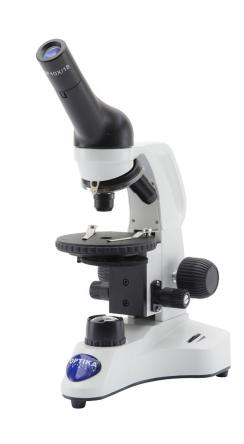
Cordless monocular microscope ideal for students and mainly primary schools, with achromatic lenses (400x), FN 18 eyepiece, finite optical system, round fixed stage and 0.3 W LED illumination with rechargeable batteries. Slim and easy to carry, it is equipped with long lasting LED illumination to provide over 20 years of use
