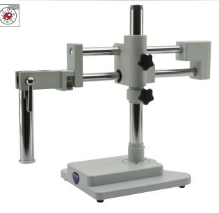
Extremely stable, long overhanging stand for observation of particularly large specimens to be matched with a focusing system and stereozoom head. Smooth horizontal and vertical movements are ensured and the head can be easily swivelled for inspection at oblique angles. In case illumination is needed, choose from the wide choice of external illuminators available.
