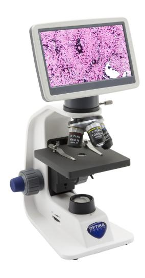
Five models of the B-150 series can be equipped with a camera and a 7" LCD screen, both in high definition. In these bundles, the normal head (supplied with the instrument) can be replaced with the digital system in a few minutes. This solution provides a system suitable for viewing specimens by several students at the same time, without removing the possibility of using the microscope in the classical way through the eyepiece.
