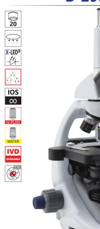
Trinocular head with IOS N-PLAN (infinity corrected) objectives, rackless stage and exclusive **X-LED**<sup>3</sup> for incredibly bright illumination.
