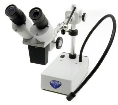
Binocular stereomicroscope ideal for large specimens, with long working distance fixed objective (2x), FN 20 eyepieces, overhanging stand and 1 W LED swiveling incident illumination. Additional objectives available for different magnifications
