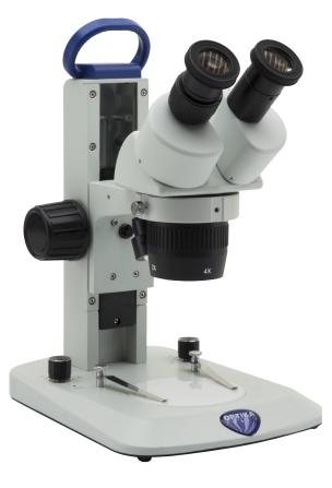
Cordless binocular stereomicroscope ideal for industrial purposes and students/amateurs to dissect and discover mainly biology and materials science in 3D, with turnable objective (2x-4x), FN 21 high eyepoint eyepieces, precision fixed arm with handle and the latest technology of EcoLED™ illumination plus rechargeable batteries. Slim and easy to carry, it is equipped with long lasting LED illumination to provide over 20 years of use
