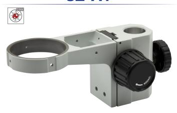
Entry-level coarse focusing to raise or lower the head to focus Coarse focusing system (76 mm head holder, 32 mm pillar) with adjustable tension for standard stereomicroscope requirements.
