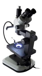
Vertical position for standard gem analysis with darkfield illumination and polarizing tecnique
