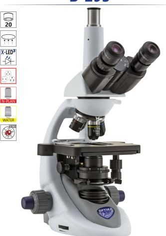
Trinocular head with N-PLAN objectives, rackless stage and exclusive **X-LED**<sup>3</sup> for unmatchable performance, powerful and uniform illumination.
