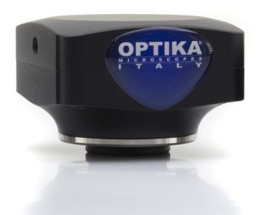
Professional yet very easy to use cameras with several resolutions, large SONY EXMOR CMOS sensor, USB3.0 connection and Global Shutter mode. Global Shutter mode can be easily thought of as a 'Snapshot' exposure mode, perfect for capturing images of moving objects and enabling 'freeze frame' capture of fast changing events, exposing each and every pixel simultaneously.
