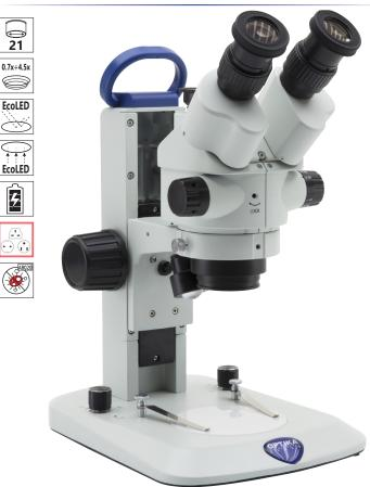
Cordless trinocular stereozoom microscope ideal for industrial purposes and students/amateurs to dissect and discover mainly biology and materials science in 3D, with 0.7x...4.5x zoom, FN 21 high eyepoint eyepieces, precision fixed arm with handle and the latest technology of EcoLED™ illumination plus rechargeable batteries. Slim and easy to carry, it is equipped with long lasting LED illumination to provide over 20 years of use
