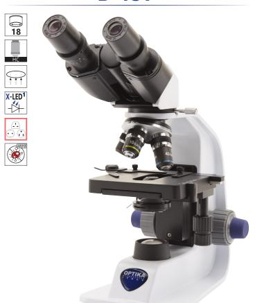
Binocular microscope ideal for students and primary schools, with four achromatic lenses (600x), FN 18 high eyepoint eyepieces, finite optical system, coaxial focusing, mechanical stage, Abbe condenser and powerful, uniform, white color temperature 1 W **X-LED**<sup>1</sup> illumination. Slim and easy to carry, it is equipped with all the main controls to start learning how to use an advanced microscope and with long lasting LED illumination to provide over 20 years of use
