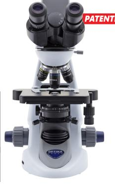
3.1 MP Built-in camera and 10.8" Windows tablet PC with N-PLAN objectives, rackless stage and exclusive **X-LED**<sup>3</sup> for unmatchable performance in illumination. Ideal for discussion group with 360° rotating tablet.
