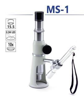
Portable monoscope ideal as multifunctional testing equipment especially for surface analysis and measurements to be used directly on the specimen. Equipped with fixed objective (10x), FN 15.5 eyepiece with crosshair and 0.3 W LED penlight for incident illumination powered by rechargeable batteries
