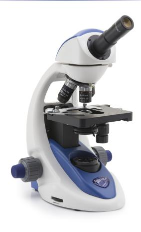
Monocular microscope ideal for teachers and secondary schools, with four N-PLAN objectives (600x), FN 18 high eyepoint, finite optical system, coaxial focusing, mechanical stage, Abbe condenser and powerful, uniform, white color temperature 3 W **X-LED**<sup>2</sup> illumination. Slim and easy to carry, yet sturdy and resistant, it is equipped with all the main controls to start learning how to use an advanced microscope and with long lasting LED illumination to provide over 20 years of use
